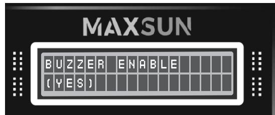
In this menu, you can switch on and off the sound of buzzer. This Alert system is very beneficial and informing, because when sun rises the controller will alert user on connected to the solar power and when sun sets down it will also alert user on disconnected from solar power. Along with this controller will also alert on over and low voltage of solar power and also when battery will low.
