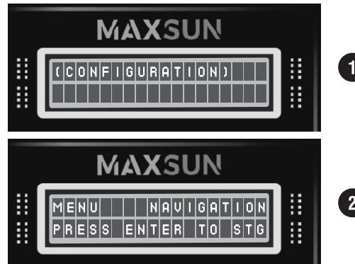
This screen is for users to customize the setting according to your desire. Users have to press the menu button to enter, after that the controller will again confirm to enter in the configuration menu; again user has to press the menu button. After entering the configuration menu, the user can change values by the long pressing the down and up buttons.
