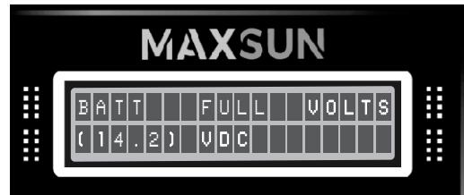
In this menu, the user can change the voltage level for the battery to fully charge.
