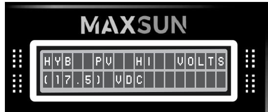
In this menu, the user can change the solar voltage level to switch off the hybrid mode.
