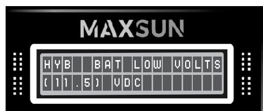
In this menu, the user can change the battery's voltage level to switch on the hybrid mode.
