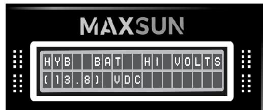
In this menu, the user can change the battery's voltage level to switch off the hybrid mode.
